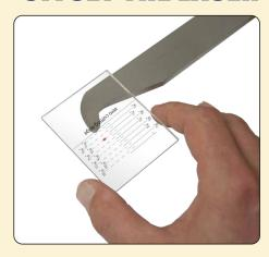
The Thickness Gauge lets you set your Turners Laser Guide for the wall thickness of your vessel. This is especially useful when you need to have a narrow or real thin vessel wall.
